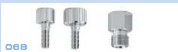
Outlet tubing nipples , 1/4 G (left) and 9/16" (middle). 1/4 G to 9/16" intermediate adaptor for connecting a 1/4G outlet flowmeter to a 9/16" inlet humidifier or nebulizer (right).
